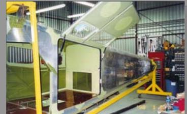
Fuselage mounted on jig with new skins and floors
